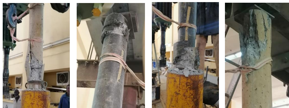
Figure 3. Mode of failures for tested columns.
